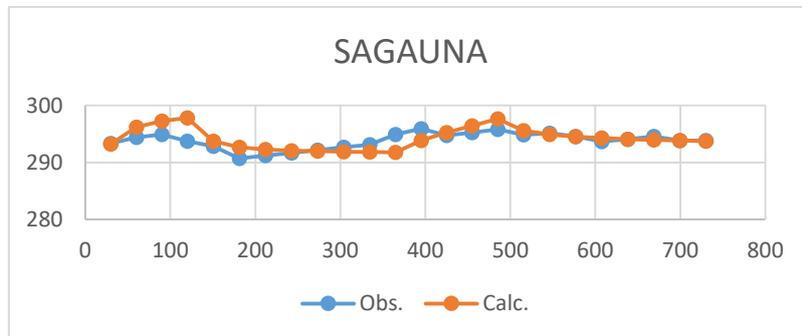
**Fig. 49g. Hydrograph of Sagauna with Observed head and Calculated head**
