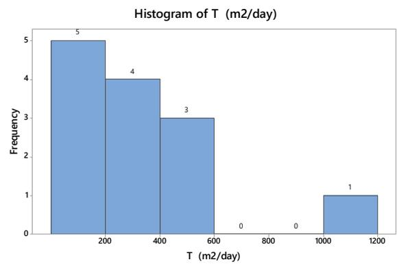
Fig.17d Histogram of Transmissivity T of bore wells
