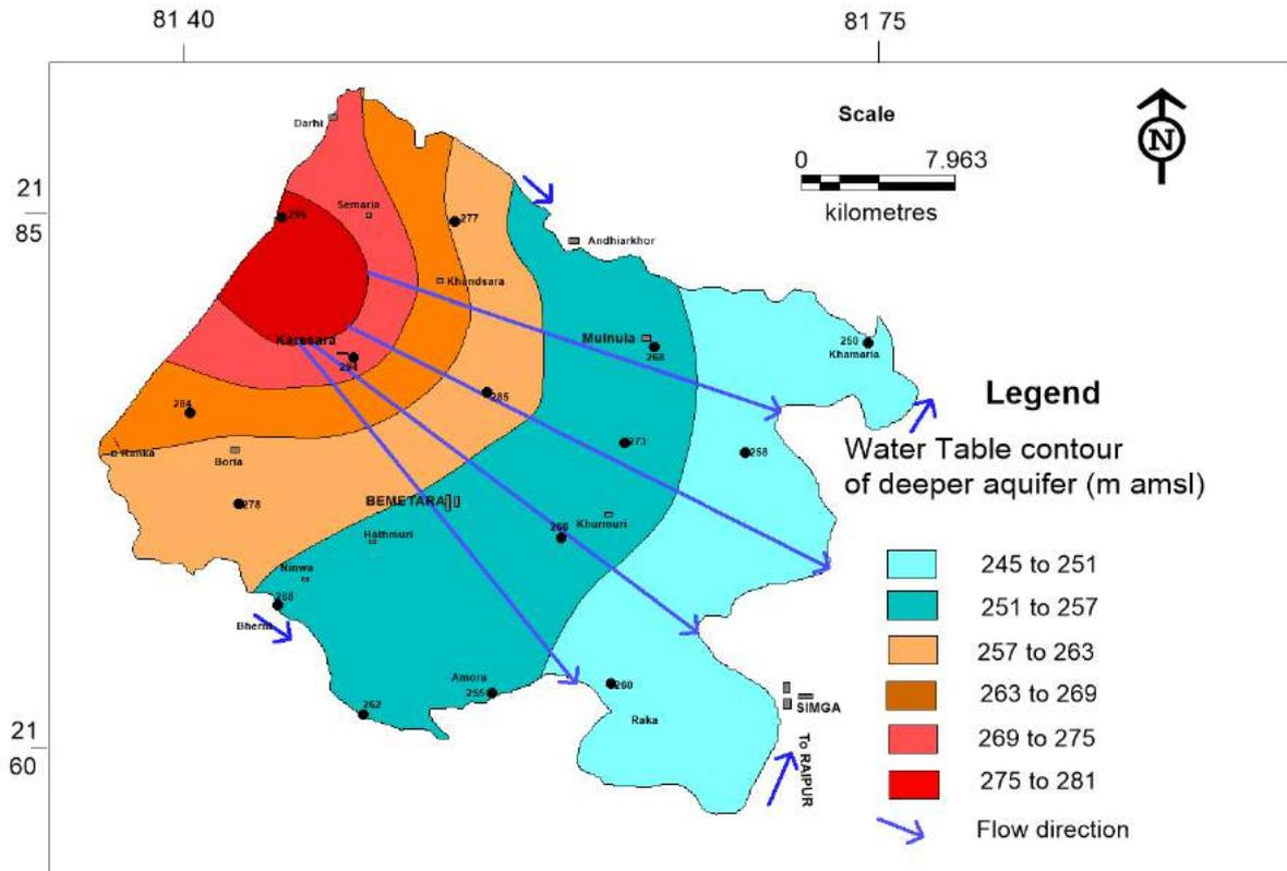
Fig.21 Water Table contour of deeper aquifer (Aquifer- II, Nov -16)
