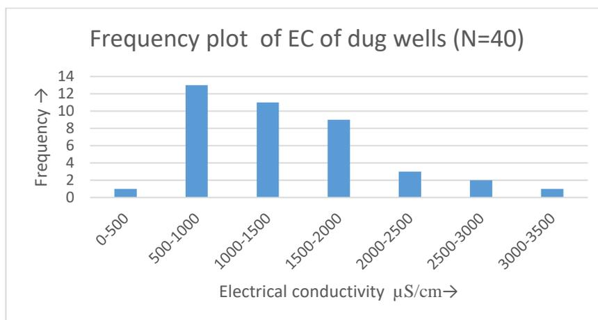
Fig. 22 Frequency plot of electrical conductivity of dug wells
