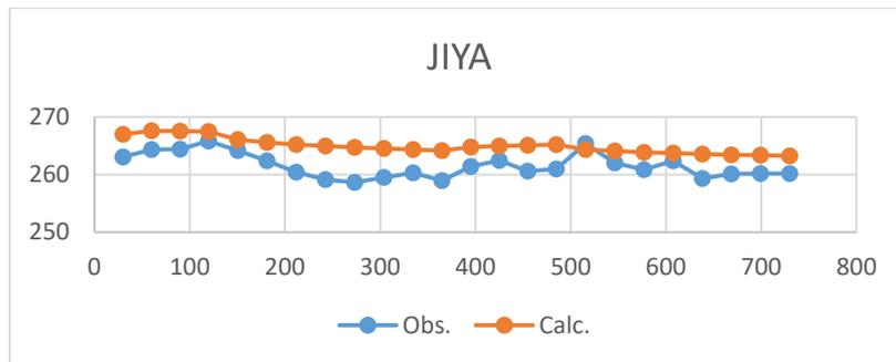
**Fig.49c. Hydrograph of Jiya with Observed head and Calculated head**
