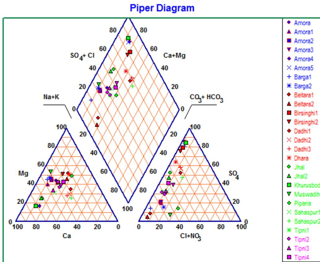
Fig.30 Piper trilinear diagram of exploratory wells
