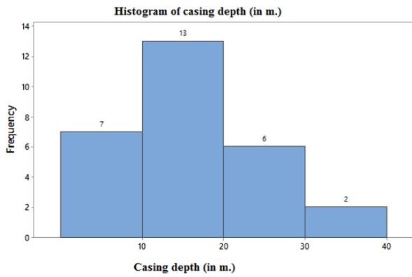
Fig.17a Histogram of casing depth of bore wells
