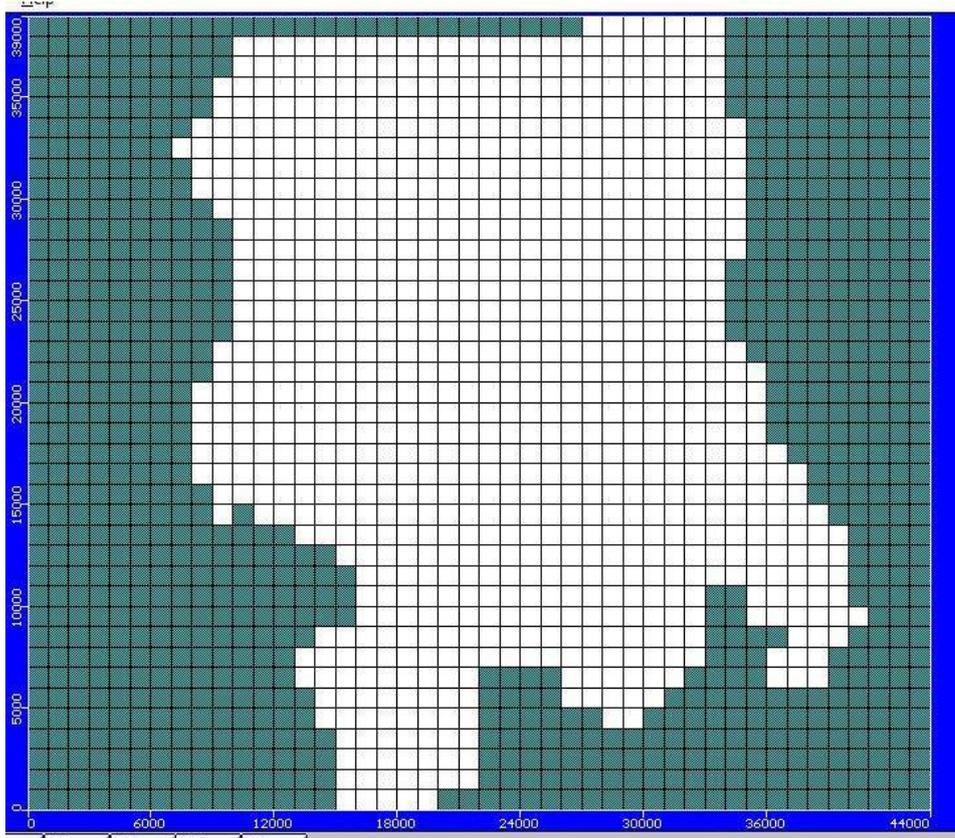
**Fig.36 Finite difference grid of the Bemetera Area**
