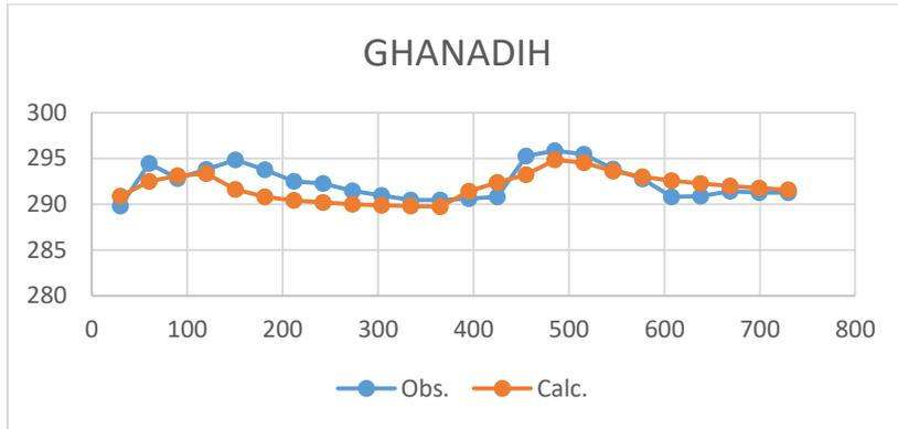
**Fig.49I. Hydrograph of Ganadih with Observed head and Calculated head**
