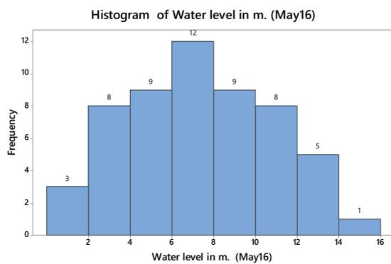
**Fig.11.1c Histogram of water level of Aquifer-I (May -16)**
