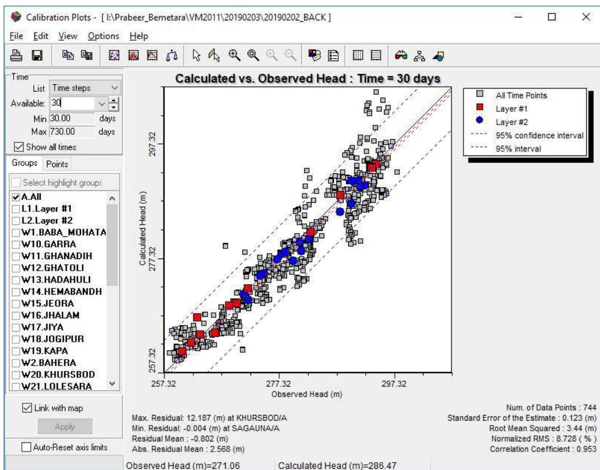
**Fig.48. Calibration Plot of Observed head versus Computed head**
