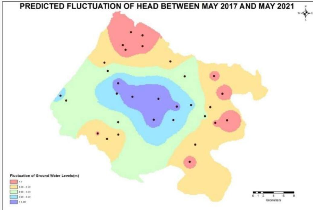
**Fig.59. Fluctuation between Ground Water Heads during Pre-Monsoon 2017 and 2021 due to Scenario III**
