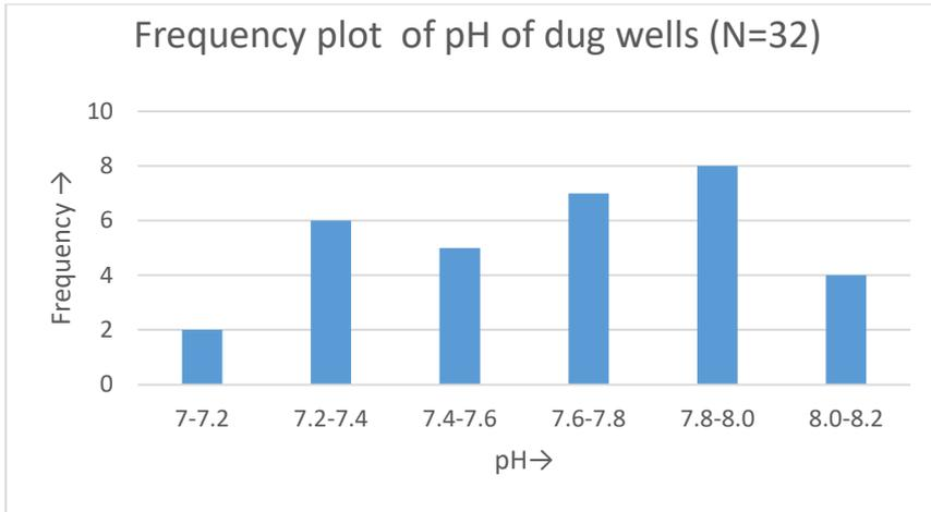
**Fig. 24 Frequency plot of pH of dug wells**
