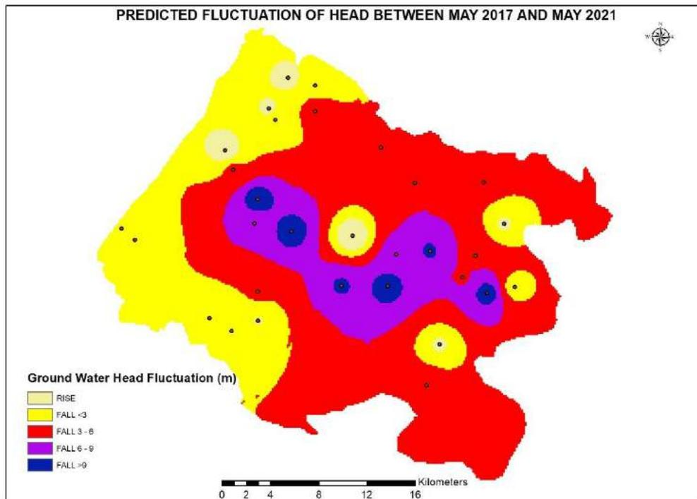
**Fig 57. Fluctuation between Ground Water Heads during Pre-Monsoon 2017 and 2021 due to Scenario II.**
