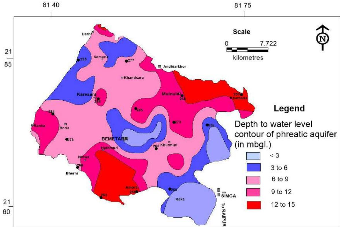
Fig.12 Depth to water level contour of phreatic aquifer (Aquifer- I, May -16)
