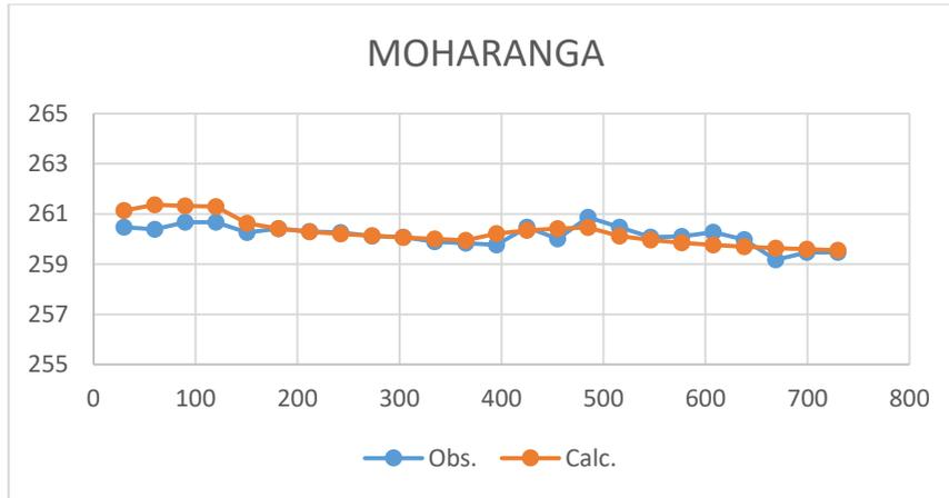
**Fig.49i. Hydrograph of Moharanga with Observed head and Calculated head**
