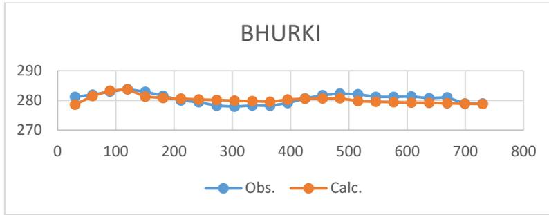
**Fig.49e. Hydrograph of Bhurki with Observed head and Calculated head**
