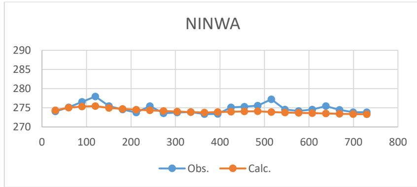
**Fig.49a. Hydrograph of Ninwa with Observed head and Calculated head**
