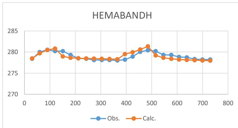
**Fig 49k. Hydrograph of Hemabandh with Observed head and Calculated head**
