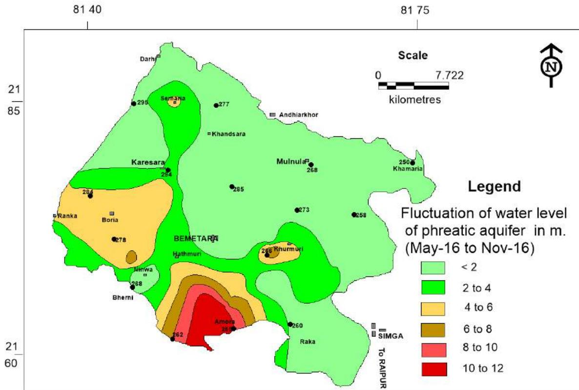
Fig.14 Water level fluctuation of phreatic aquifer (Aquifer- I, 2016)
