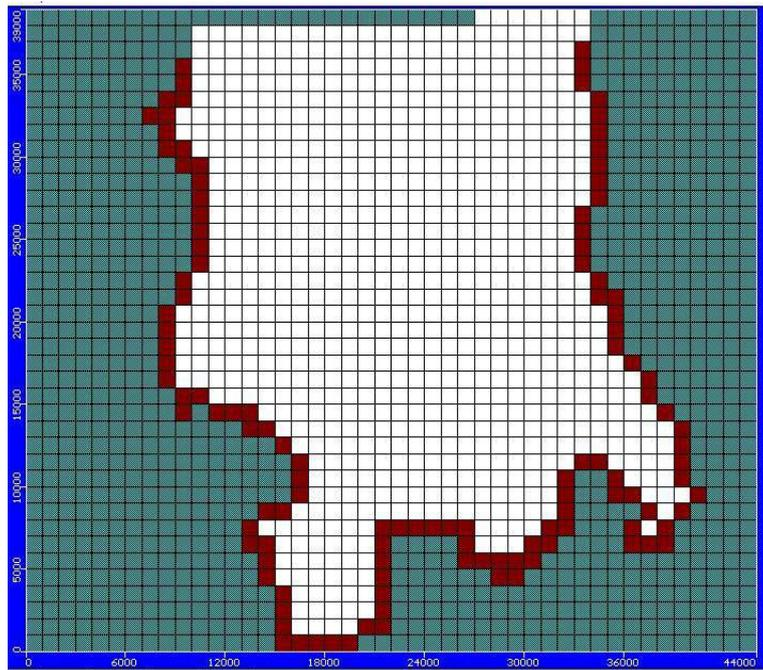
**Fig. 38 Constant Head Boundaries simulated in the Bemetara Area**
