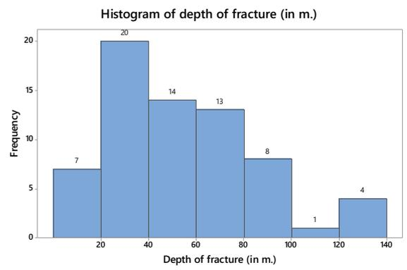
Fig.17b Histogram of depth of fractures of bore wells
