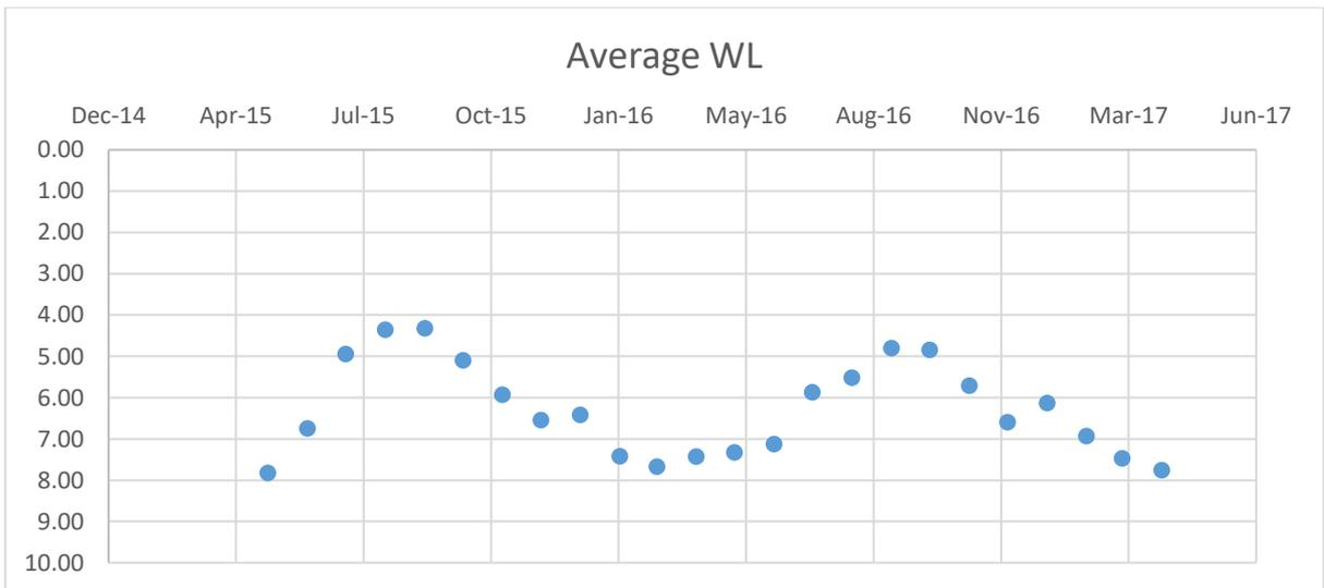
**Fig. 11.1f. Plot of average water level of dug wells**
