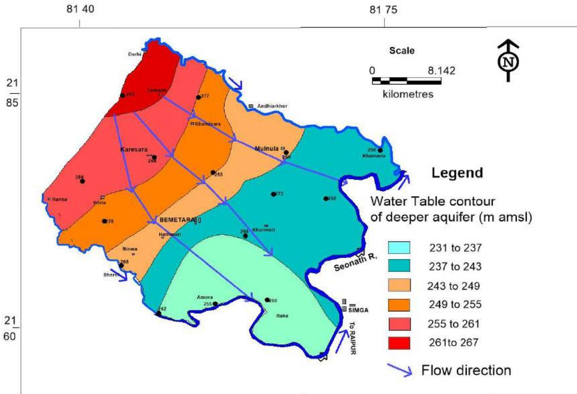
Fig.20 Water Table contour of deeper aquifer (Aquifer- II, May -16)
