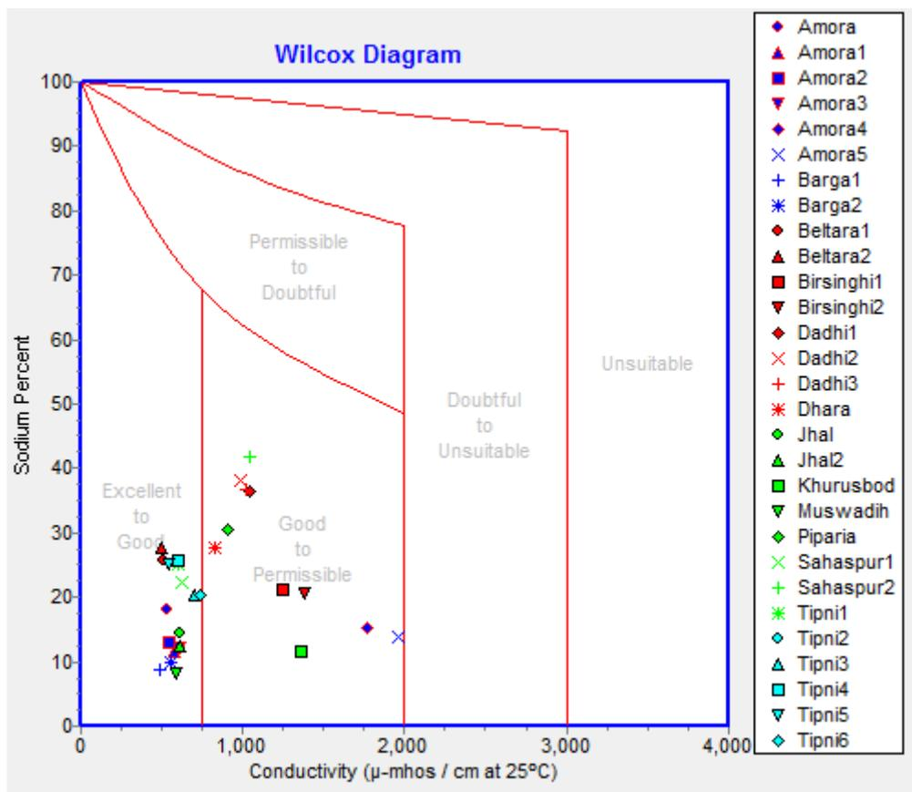
**Fig.32 Wilcox diagram of exploratory wells**
