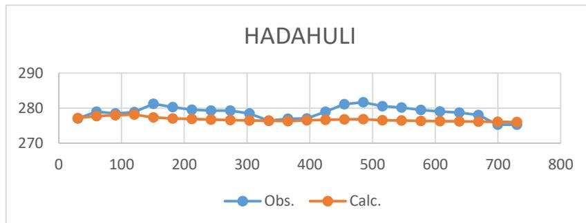
**Fig.49d. Hydrograph of Hadahuli with Observed head and Calculated head**
