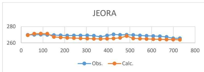
**Fig 49j. Hydrograph of Jeora with Observed head and Calculated head**
