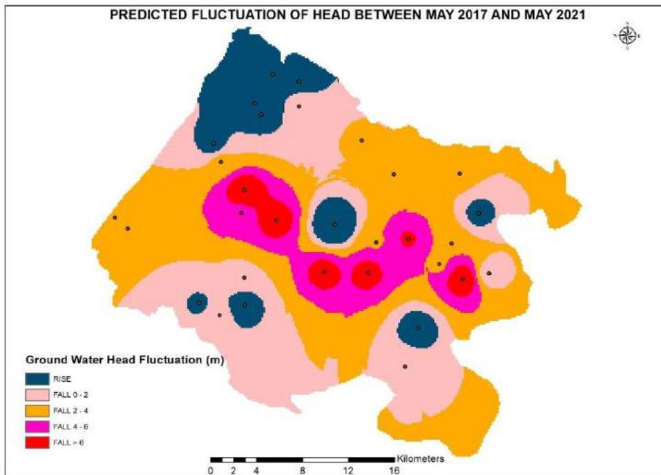
**Fig.55. Fluctuation between Ground Water Heads during Pre Monsoon 2017 and 2021 due to Scenario I.**
